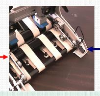
Our Patented paper guide extensions guide the document right into the gripper, eliminating extra components and touchy photo eye adjustments!
